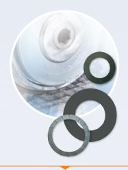
ADT's Resin-bond Blades are manufactured through a unique proprietary molding process. When cutting hard and brittle materials, the edge of the blade wears out at a controlled rate exposing new diamonds to constantly sharpen the blade and thus achieve highly accurate kerf, outstanding yield and exceptional blade life.
