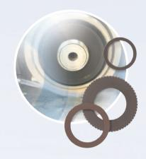
In a unique close-mold sintering process, diamond grit size, diamond concentration and metal binder are optimized to meet the precision and blade life requirements of your specific application. The metal binder provides a very stable, stress-free blade matrix and can be custom tailored to meet the required hardness and load resistance for dicing a variety of applications.
